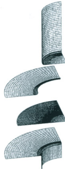
Figure 8.2 Exploded view of mesh used to simulate cylindrical cup draw (Harpell, 1997)
